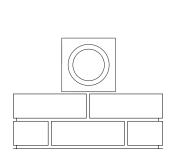
Build up brick work to desired height and set paper ring in place
